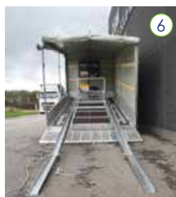
The BM53000 wheel play detector unit is rolled down using the electrical winch. Rails are then moved to the top of the transport rail system whereafter the BM20200 mobile brake tester is rolled down using the electrical winch.
