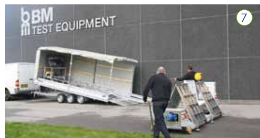
Both the BM20200 and BM53000 are supplied with small wheels so one person can easily place the equipment on the preferred location for vehicle testing.
