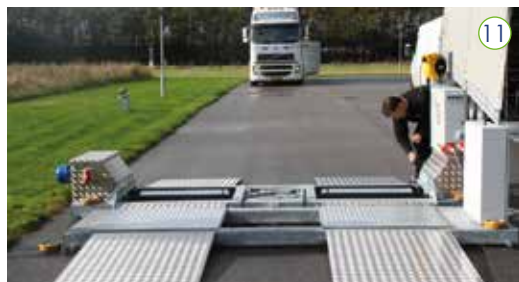
Final adjustments before vehicle is called forward. Approximate setup time for two persons is 5-10 minutes.
