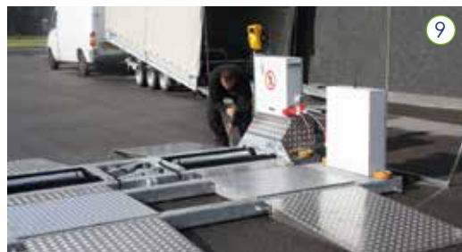
The equipment has strong feet with high resistant contact path. All feet can be adjusted in height to offset uneven ground.
