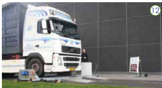
First axle of the vehicle is being tested on the BM20200 mobile roller brake tester.
