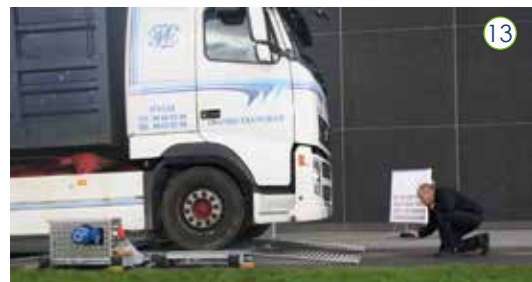
The vehicle is driven forward so the first axle is on top of the BM53000 wheel play detector.
