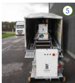
The BM53000 wheel play detector unit is rolled down using the electrical winch. Rails are then moved to the top of the transport rail system whereafter the BM20200 mobile brake tester is rolled down using the electrical winch.
