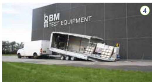
Special unload rails are placed and equipment is rolled down using the integrated electrical winch.
