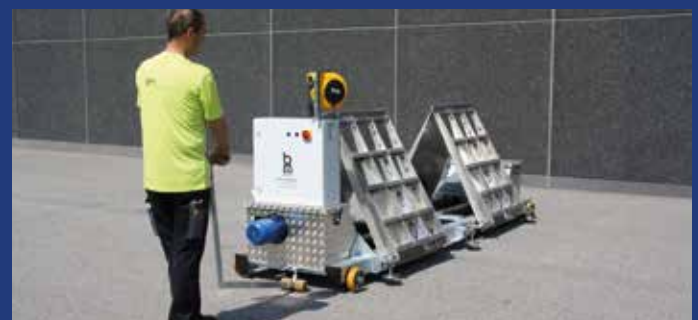
Both the BM20200 brake tester and the BM53000 wheel play detector can easily be towed to their correct positions or stored by one person.
