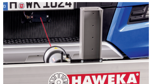
SAD4000 camera setting on the ACC sensor
